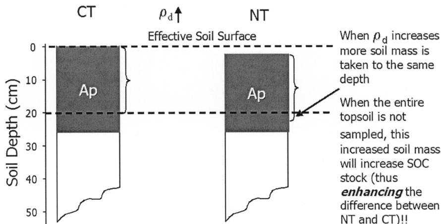
**Fig. 3.** Schematic illustrating that sampling to fixed depths in no-till and conventional tillage could inflate rates of SOC change in favor of the no-till system.
